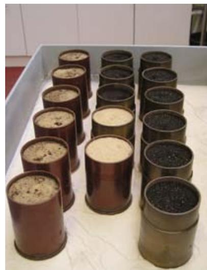
**BRINGING SAMPLES TO EQUILIBRIUM ON THE TENSION TABLE – This is required to establish the porosity levels and water retention for each sample**
