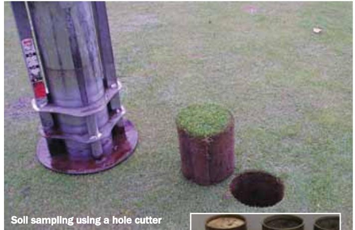
Soil sampling using a hole cutter
